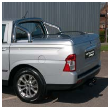
Top up cover (flat glassfibre cover, hinged to offer flexible opening options) £1,655.00
